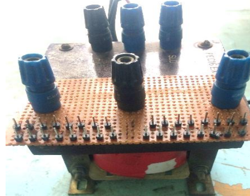
Fig.9. Practically designed transformer 230/24v
