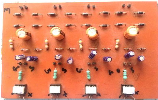
Figure.7. PCB designed Gate driver circuit
