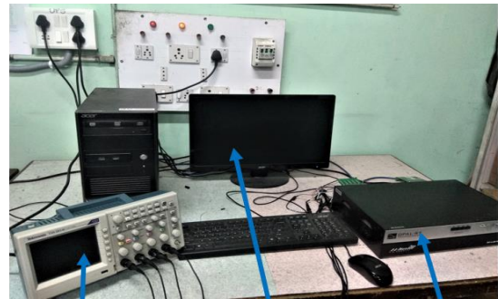
Four Channel DSO (Tektronix, TDS 2014C) Host PC with RT Lab Environment OPAL-RT (OP-4503)
