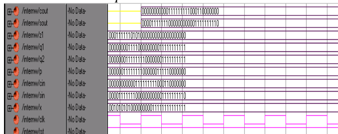
Fig. 9.3 Internal Cell Output
